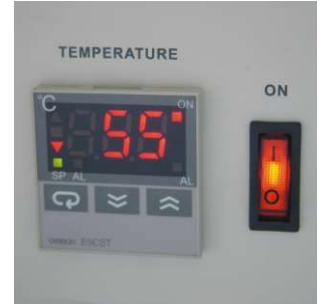
Heating device available for increasing tape adhesiveness.
