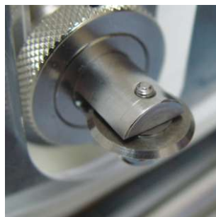
Heavy-Duty roller type harden steel cutter.
